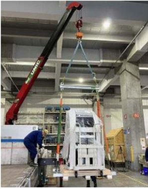
SLINGS DIRECTLY CONNECTED TO HOOK ON TOP WITH LIFTING BARS UNDER THE PALLET
