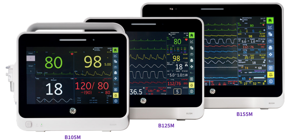
Choice of 10-, 12- or 15-inch capacitive touch screen displays
